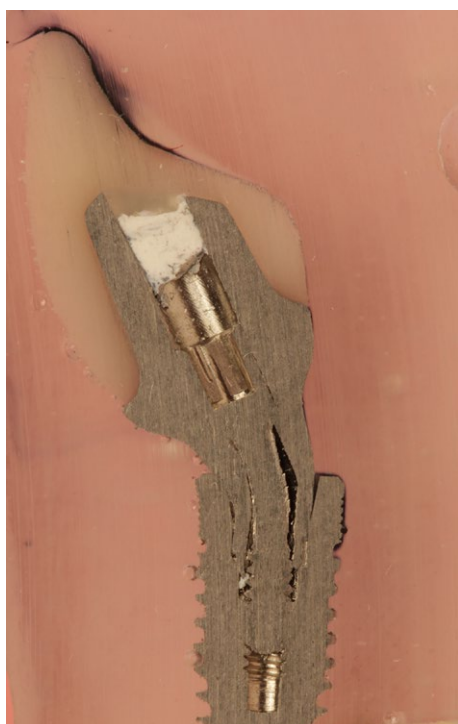
FIGURE 3 A sectioned specimen of group Ti, showing plastic deformation of the screw and the abutment without any fracture
